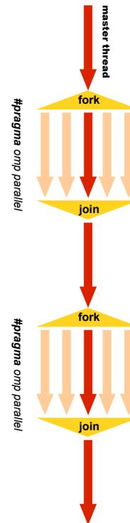
Figure 4: OpenMP is based on a fork-join model
