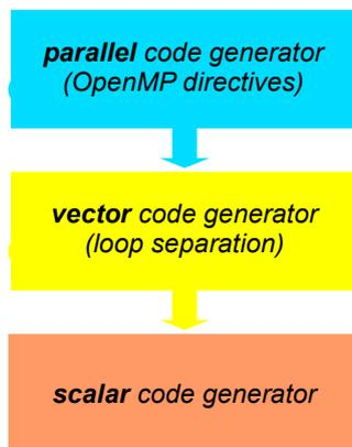
Figure 3: Faust's stack of code generators
